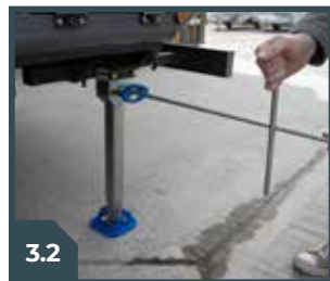
WIND CORNER STEADY TO GROUND LEVEL
