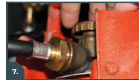
TURN OFF GAS BOTTLE VALVE WHEN PACKING DOWN
