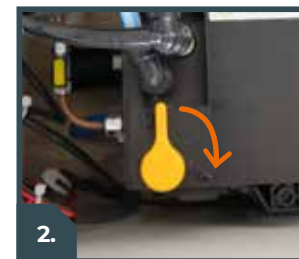
2. TURN THE FLOW VALVE TO EMPTY UNIT
