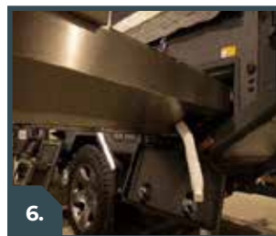
WASTE PIPE EXTENDED
