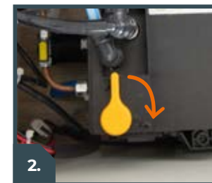
2. TURN THE FLOW VALVE TO EMPTY UNIT
