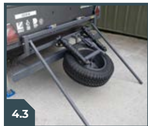
REST BED LEGS ON THE GROUND
