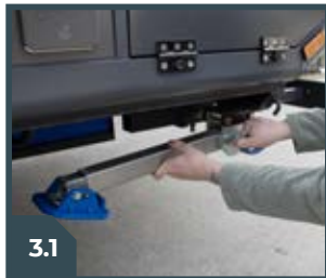
RELEASE BLUE HANDLE TO LOWER STEADY
