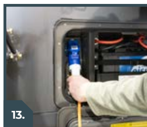
DISCONNECT THE HOOK-UP CABLE
