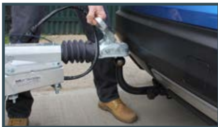
LIFT THE COUPLING HANDLE
