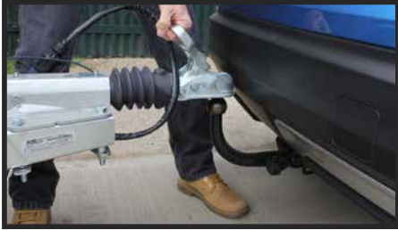
LIFT THE COUPLING HANDLE
