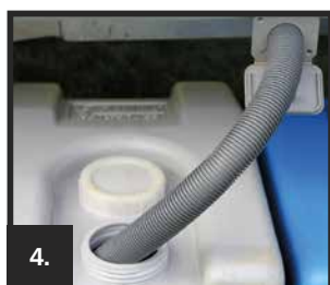
4. WASTE PIPE CONNECTION
