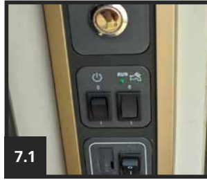
7.1 HEATER ISOLATION SWITCH
