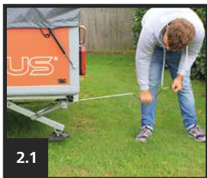
WIND DOWN CORNER STEADY
