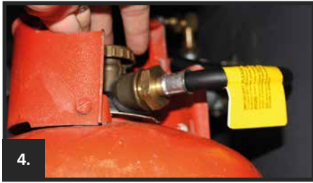
OPEN THE VALVE ON THE BOTTLE
