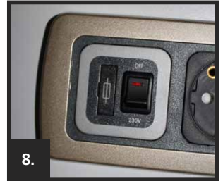
8. SWITCH OFF HEATER ISOLATION SWITCH
