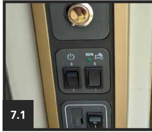
7.1 HEATER ISOLATION SWITCH
