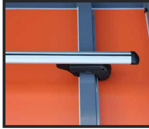
ROOF BAR FEET, CLAMP OVER THE GRIP RAILS FITTED ON THE ROOF LID RIBS.
