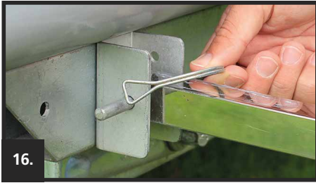
16. REMOVE THE REAR BED SUPPORT LEGS
