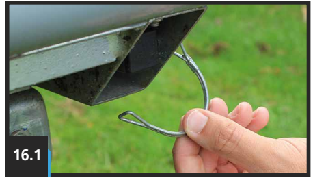
16.1 D-PIN SECURES BED SUPPORTS
