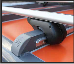
ROOF BAR FEET, CLAMP OVER THE GRIP RAILS FITTED ON THE ROOF LID RIBS.
