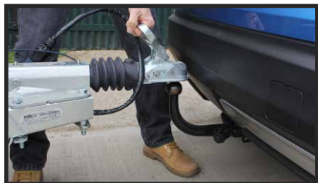
LIFT THE COUPLING HANDLE
