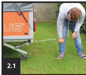
WIND DOWN CORNER STEADY
