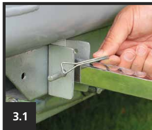
SECURE BASE OF LEG WITH D-PIN
