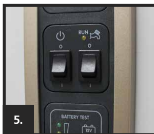
5. MAIN & RUN SWITCH ON
