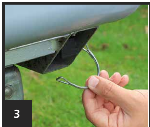
REMOVE THE D-PIN TO RELEASE LEG
