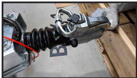
STANDARD LOCKING COUPLING
