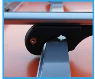
ROOF BAR FEET, CLAMP OVER THE GRIP RAILS FITTED ON THE ROOF LID RIBS.
