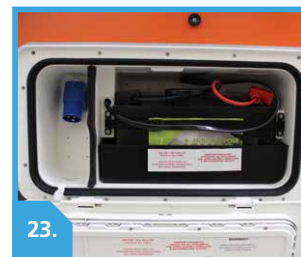
CHECK LEISURE BATTERY IS SECURE & BATTERY BOX IS LOCKED
