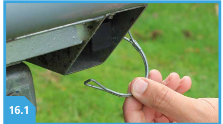
16.1 D-PIN SECURES BED SUPPORTS
