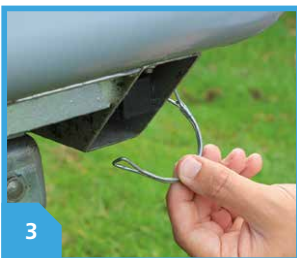
3 REMOVE THE D-PIN TO RELEASE LEG
