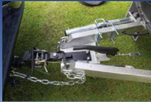
The Air OPUS Off-Road is built for serious off-the-beaten-path camping with its independent trailing-arm suspension and twin shock absorbers (far left) and Lock 'N' Roll articulating coupler with three-way movement (left). (Below) Next stop: Southern California's Zuma Beach for some standup paddleboarding. The side-pivoting cargo rack is rated for 700 pounds and lifts easily out of the way when setting up the OPUS.
