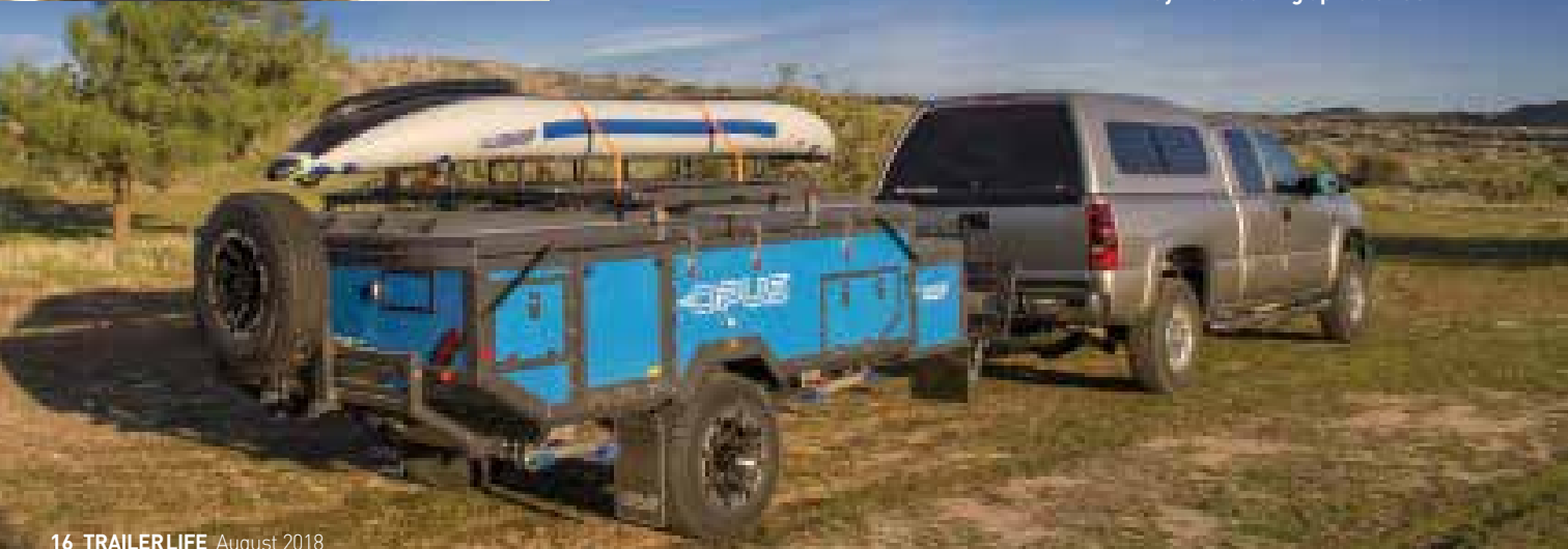
The Air OPUS Off-Road is built for serious off-the-beaten-path camping with its independent trailing-arm suspension and twin shock absorbers (far left) and Lock 'N' Roll articulating coupler with three-way movement (left). (Below) Next stop: Southern California's Zuma Beach for some standup paddleboarding. The side-pivoting cargo rack is rated for 700 pounds and lifts easily out of the way when setting up the OPUS.
